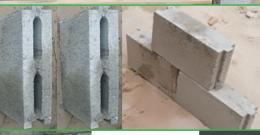
Partitioning Interlocking Hollow Block is 400mm x 100 x 100mm
